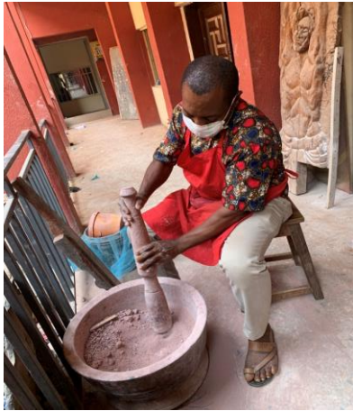
Plate XI: Showing the Researcher Pounding the Clay Used for the Refractory. Photo by Gaius Ikenna
