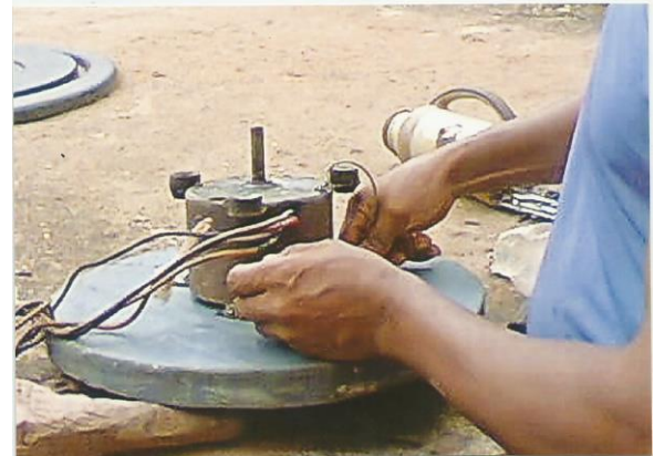
Plate VI: Mounting of the Motor Fan blade on the cover part. Photo by Ikenna.
