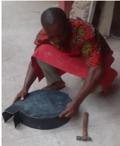
Plate V: The researcher forging the Blower Casing Source: photo by Gaius Ikenna
