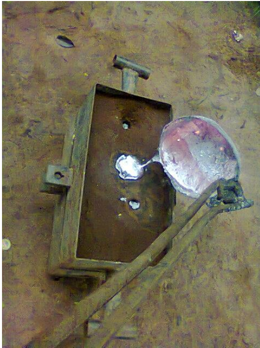
Plate XIII: Pouring the Molten Metal into the Already Made Mould. Source: Photo by Gaius Ikenna
