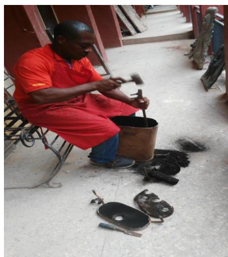
Plate VIII: The Researcher Shown Cutting and Removing the Exhaust compartments Photo by Gaius Ikenna
