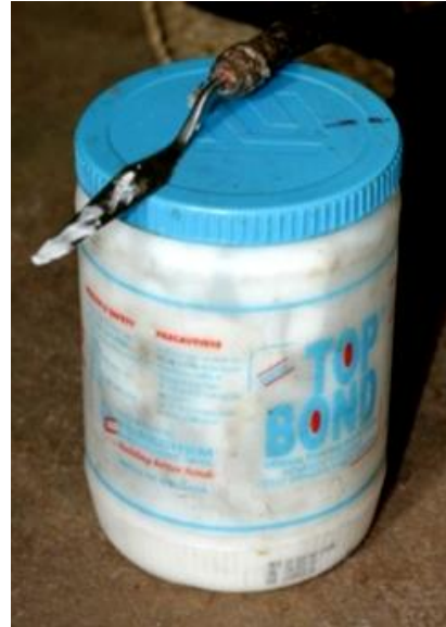
Plate 20: Top bond adhesive mixed with saw dust was used in fastening the appropriated materials. Photo source: Job Ukwa (2020)
