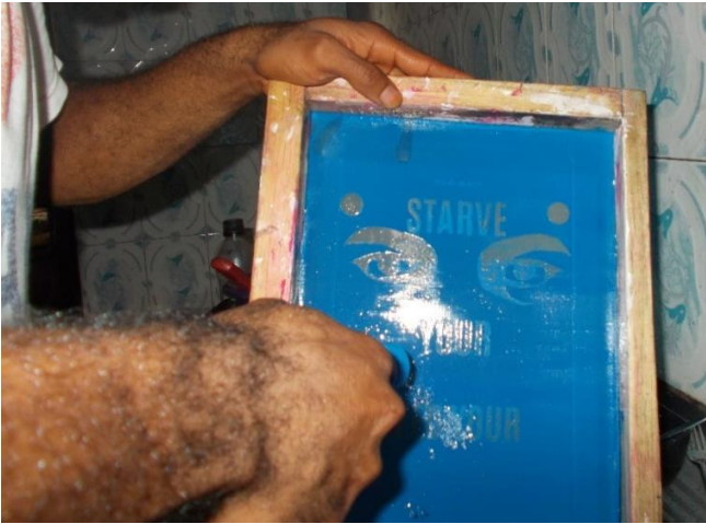
Plate 11: Registered image being developed, fixed and washed with water on screen. © The researchers
