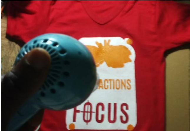
Plate 13; Printing of first few colours and quick drying to enable successive printing. © The researchers
