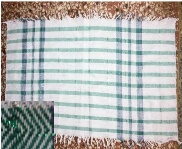
Plate 2: Reversed Twill weave fabric produced by the author Medium: 100% cotton warp and weft. 2012.
