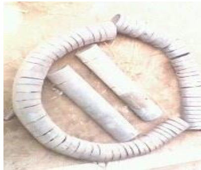
Plate. 8 Rings fold to achieve circular shape
