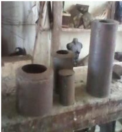
Plate 10: Cylindrical shapes formed from welding
