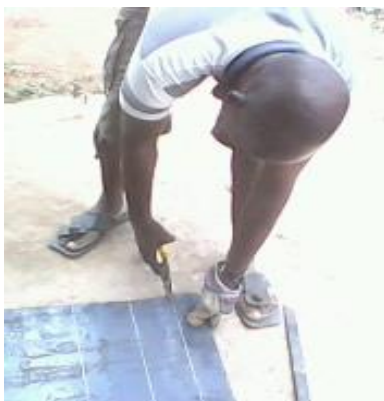
Plate. 3. Cutting of metal into parts
