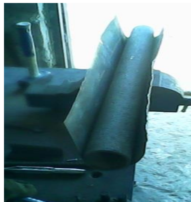
Plate. 5. Folding of metal plate to produce forms
