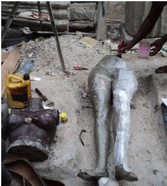
Plate 8: Taking the Mould in Resin and Fibre Matt. (FRP). Photos: Anyaegbunam L.U, 2012
