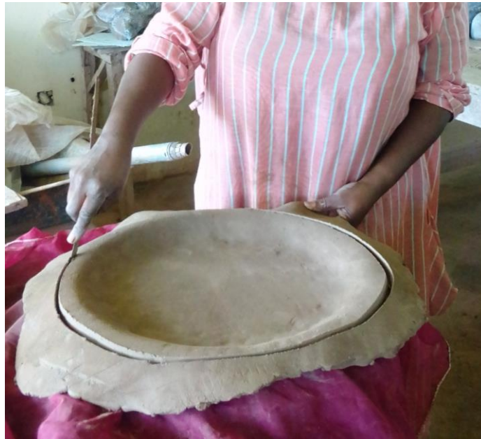
Plate 5 : Making of tray using casting method of production
