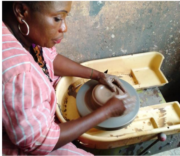
Plate 3: Pulling of the Centered Clay
