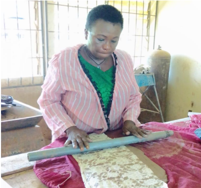
Plate 9: Pressing floral lace pattern on the slab
