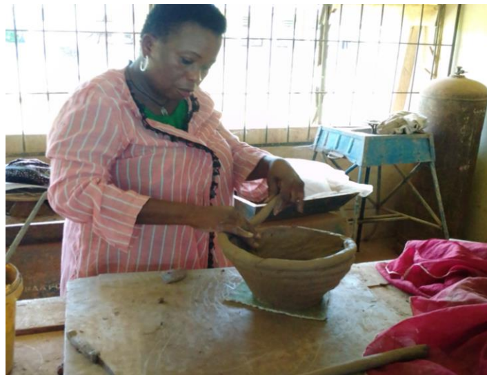
Plate 6 : Building the wall of the planter with clay coils
