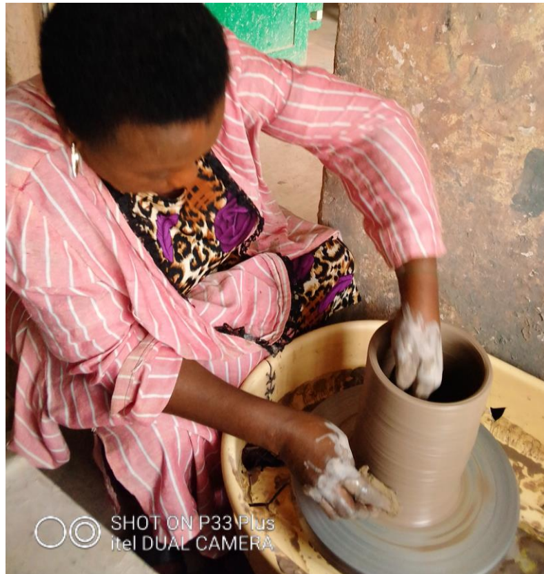
Plate 2: Centering of Clay
