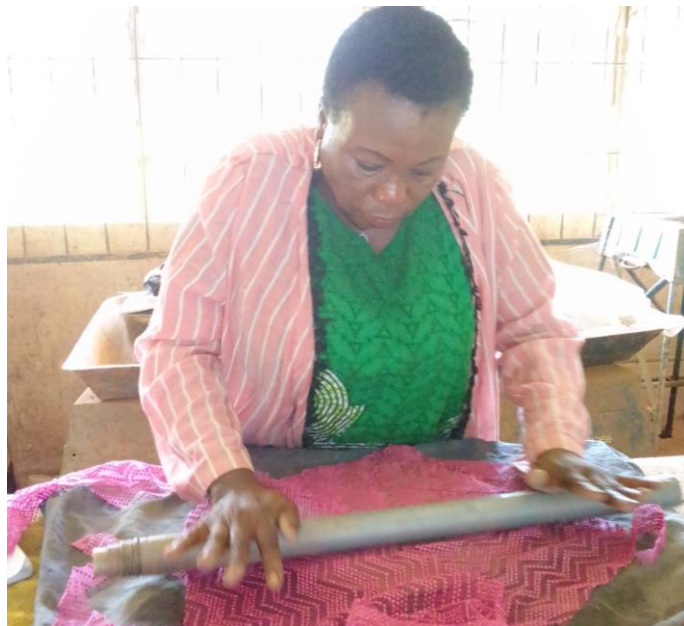
Plate 8: Pressing zigzag lace pattern on the slab
