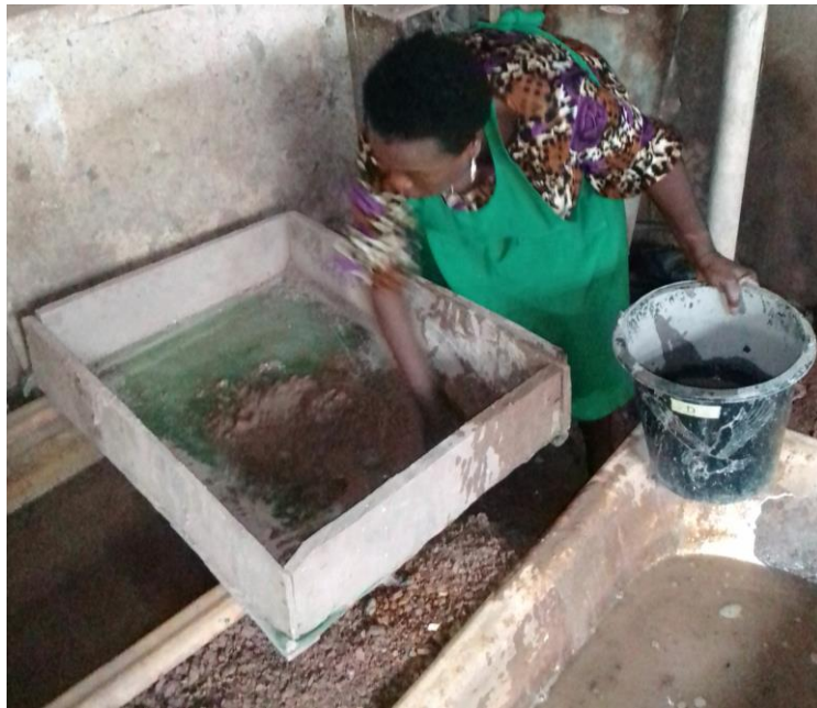
Plate 1: Modern /Studio method of sieving clay
