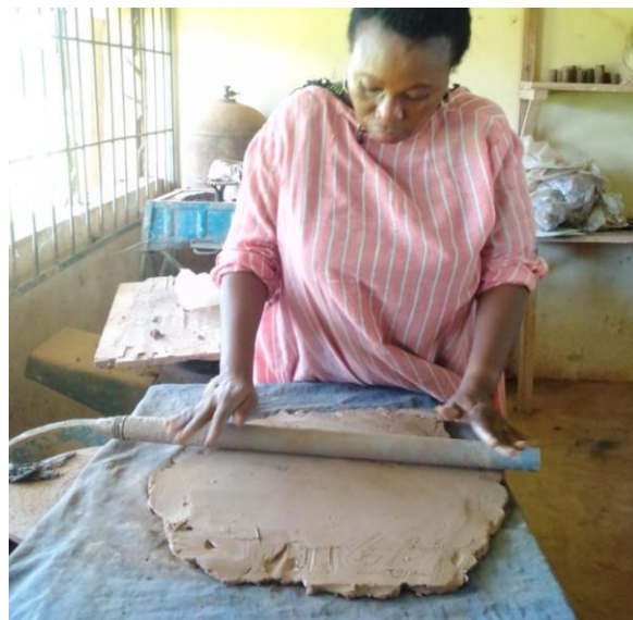
Plate 4: Rolling of slab
