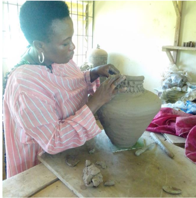
Plate 7: Forming the neck of the planter
