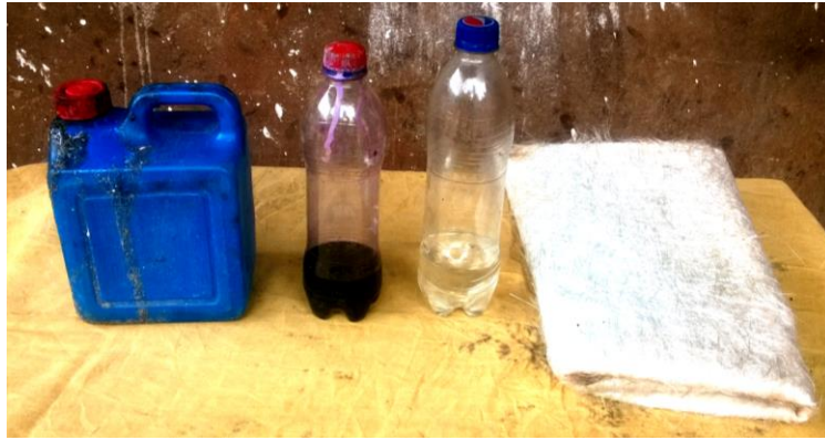
Plate 2. Polyester Resin, Accelerator, Catalyst and Fibre Mat (from left to right)
