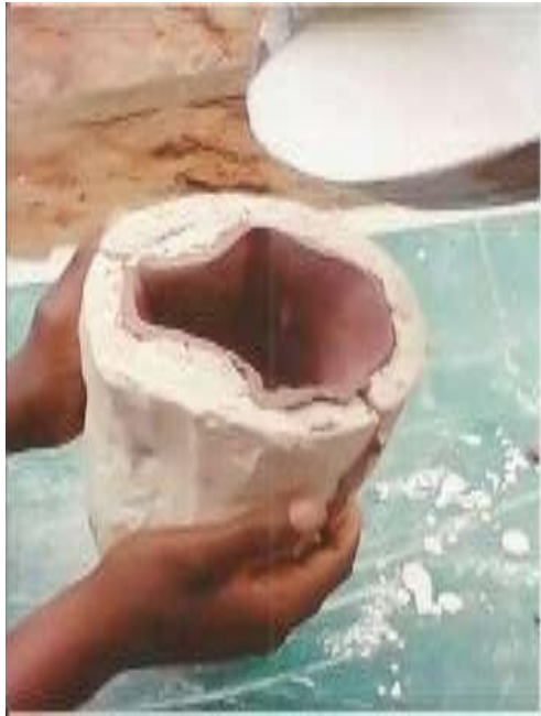
Plate 4: Showing the researchers casting core of a mould used for lost clay technique
