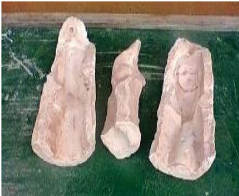
Plate 5: Showing in Pieces the two Half Halves and Core of the Mould
