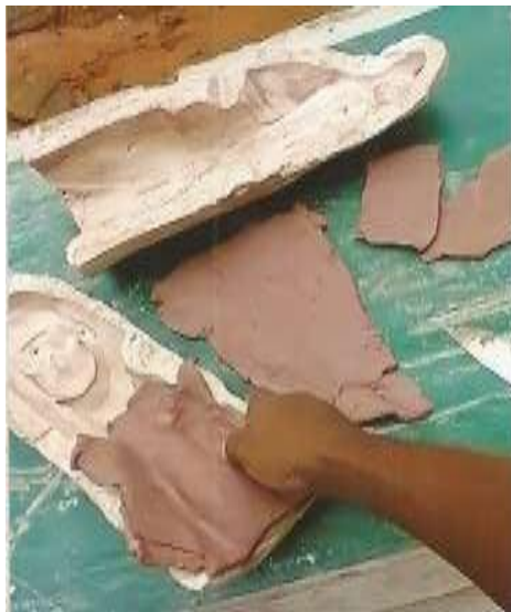
Plate 3: Showing Slabs of Clay and Process of obtaining the Core for the Pop Plaster Mould
