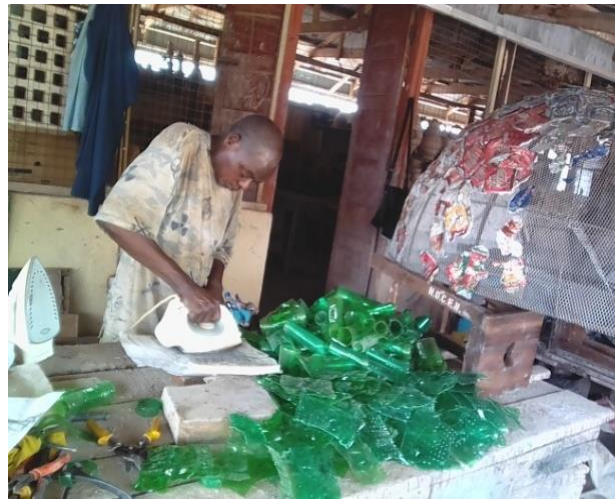
Plate 2: Slicing and Flattening Plastic Beverage Containers © The researcher, 2018
