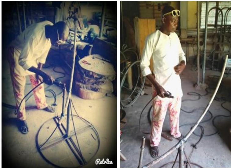
Plate 12 and 13: Designing and Welding the Globe Stand. © The researcher, 2018
