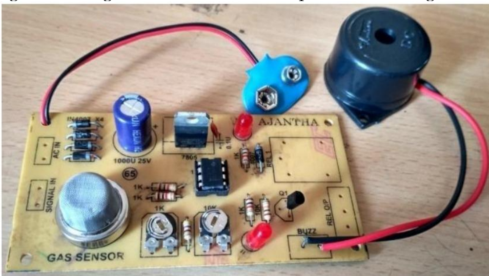
Figure 5: LPG leakage detection and alert system
