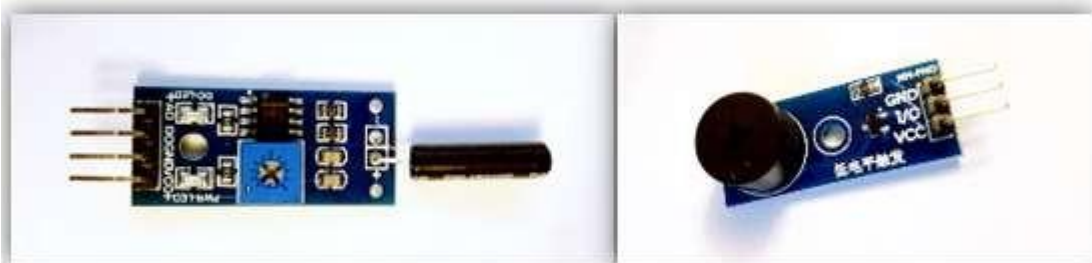
Fig. 13. Seismic Sensor (left) and buzzer (right)
