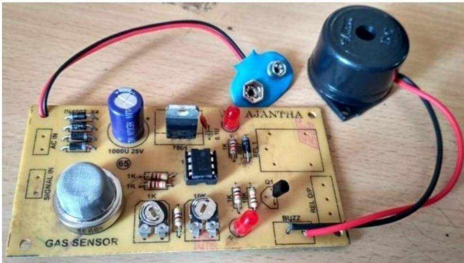
Figure 5: LPG leakage detection and alert system
