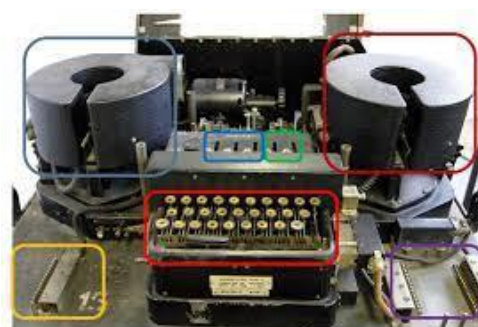
Fig 7: The British 'Typex' (Chang, 2012).
