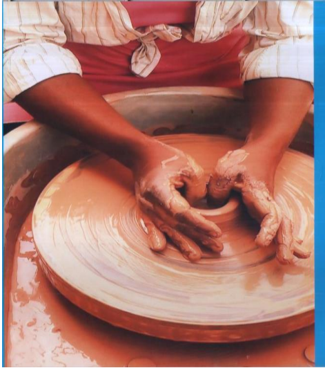
Plate 4: Opening up the Clay
